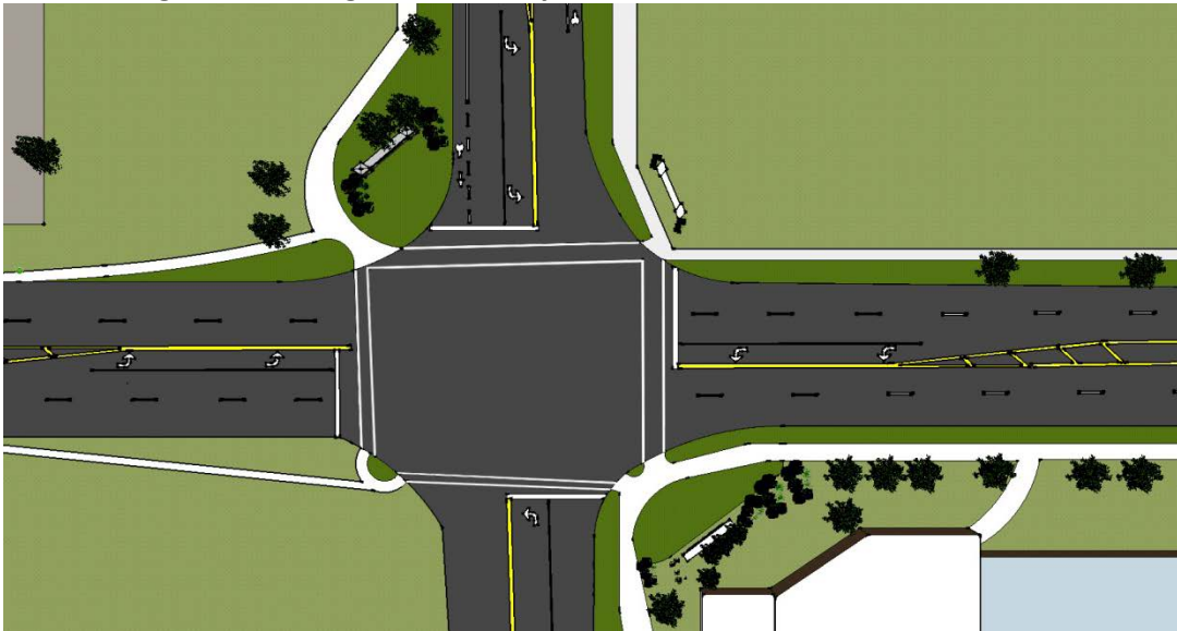
Figure 6: Existing Schematic Layout at the Race/Windsor Intersection
