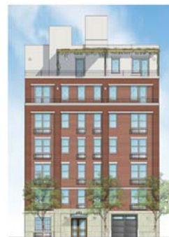
Parking is on ground floor, but is screened and not visible in the façade zone
