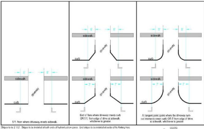
Stripes to be 21 X.2. Stripes to be installed at both ends of hydrent yallow zones. End stripes to be installed at border of No Parking Here. To Corner zones. Distance from ourb to inside edge of stripe is 7.6°, therefore, 4° wide stripe will run from 7.6° to 8°0° marks. Distance to line face is 50° to the cutside edge, therefore, a 4° wide stripe will run from 5.0° to 5°4°.
