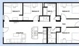
Interior Unit Typical for 1st, 2nd, 3rd, and 4th Floors Area = 1,180 GSF
